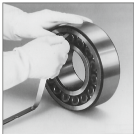
Fig. 1: Checking bearing clearance with bearing on bench.
