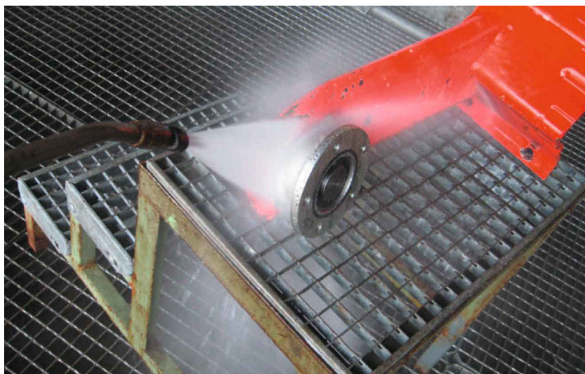
Figure 3: Tested using a water jet for 200 hours
