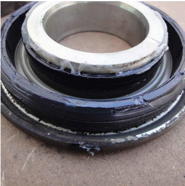
No dirt was able to get through the cassette seal. The seal is in outstanding condition
