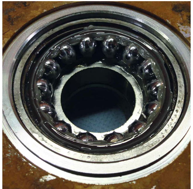
Once the bearing had been dismantled, no dirt was found inside the bearing or in the lubricant
