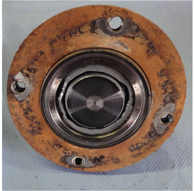
The picture shows that no contamination or rust is present beyond the O-ring
