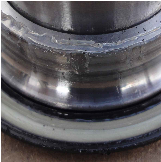
There is no sign of damage or wear to the raceways
