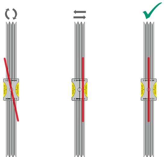
The LAB-Set units are very easily mounted on the pulleys. The spring action probe finds the centre of the belt groove. The built-in industrial magnets snap the units to the pulley in a perfect fit. Optional equipment makes it possible to align timing belt driven machines.
