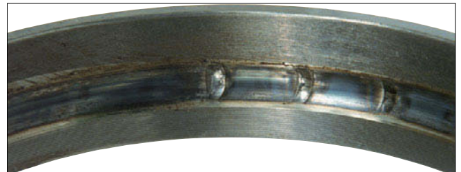
Part: Outer ring of an angular contact ball bearing Symptom: Raceway discoloration; melting occurs at ball pitch intervals Cause: Excessive preload
