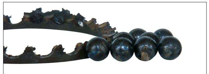
Part: Balls and cage of an angular contact ball bearing Symptom: Cage is damaged by melting; balls become discolored and melted Cause: Excessive preload
