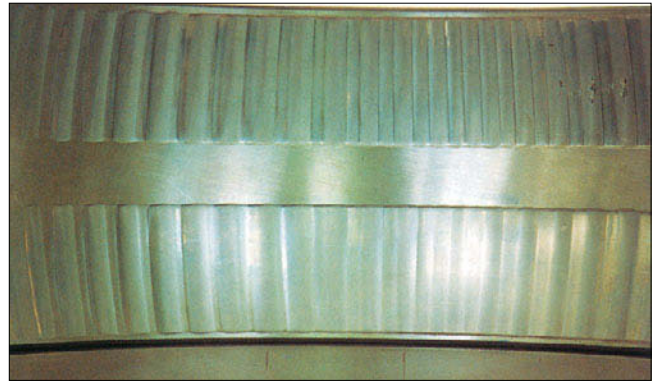
Part: Outer ring of a spherical roller bearing Symptom: Wear having a wavy or concave-and-convex texture on loaded side of raceway surface Cause: Entry of foreign matter under repeated vibration while stationary
