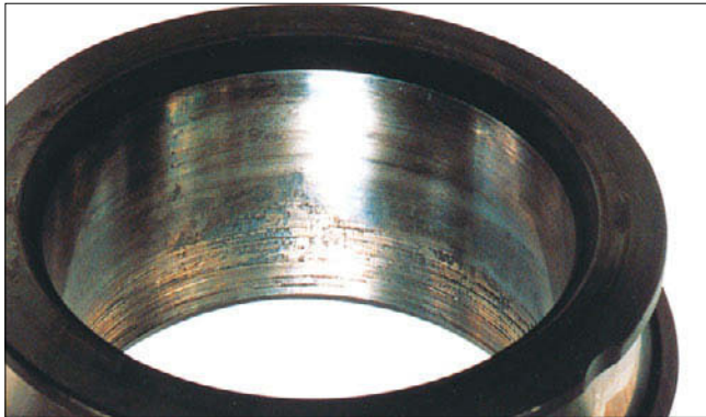
Part: Inner ring of a spherical roller bearing Symptom: Creep accompanied by scoring of bore surface Cause: Insufficient interference
