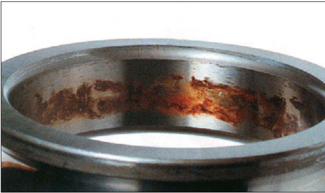
Part: Inner ring of a deep groove ball bearing Symptom: Fretting occurs on the bore surface Cause: Vibration
