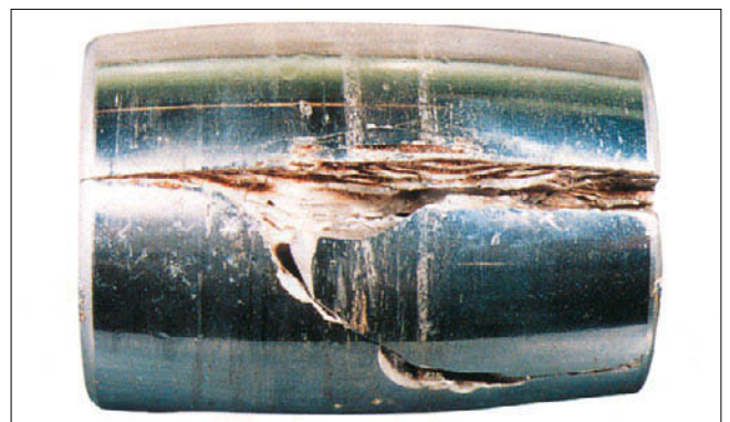
Part: Roller of a spherical roller bearing Symptom: Axial cracks occur on rolling surface
