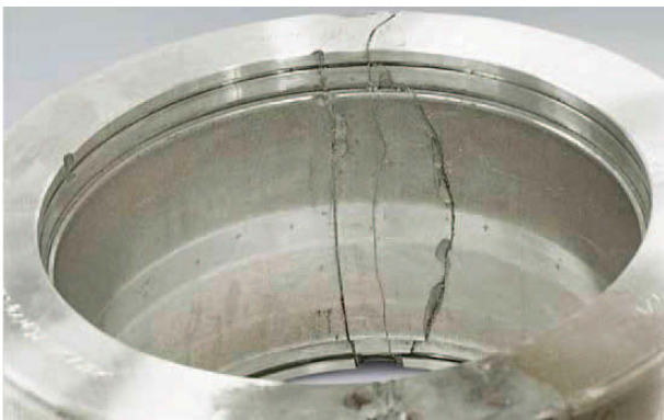
Photo 6.5 Part: Raceway surface of outer ring in Photo 6.4 Symptom: Outside surface crack developing on the raceway
