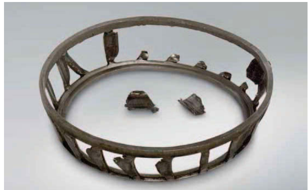
Photo 7.4 Part: Cage of a tapered roller bearing Symptom: Pillar fractures of pressed-steel cage
