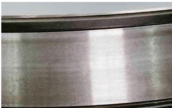
Photo 8.3 Part: Inner ring of a tapered roller bearing Symptom: Small and large indentations occur over entire raceway surface Cause: Debris caught in the surface
