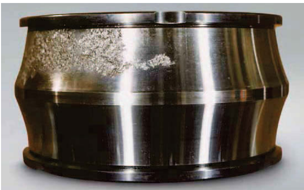
Photo 1.9 Part: Inner ring of a spherical roller bearing Symptom: Flaking of only one row of raceway Cause: Poor lubrication
