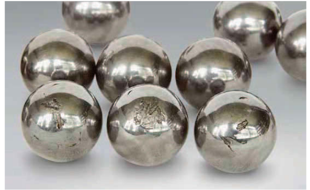
Photo 1.6 Part: Balls of Photo 1.4 Symptom: Flaking of ball surface Cause: Dents due to shock load while stationary
