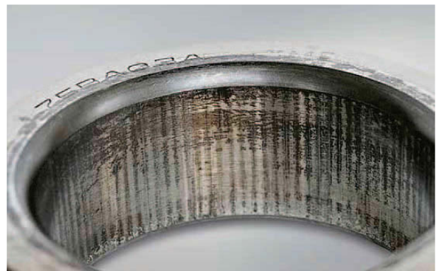
Photo 11.2 Part: Inner ring of an angular contact ball bearing Symptom: Notable fretting occurs over entire circumference of bore surface Cause: Insufficient interference fit
