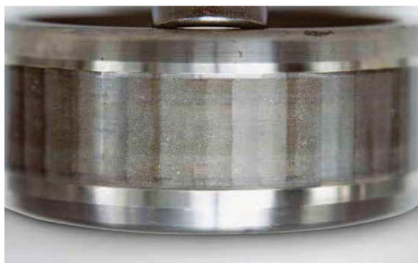
Photo 10.1 Part: Inner ring of a cylindrical roller bearing Symptom: Many pits occur due to electrical corrosion and wave-shaped wear on raceway surface Cause: Electrical corrosion
