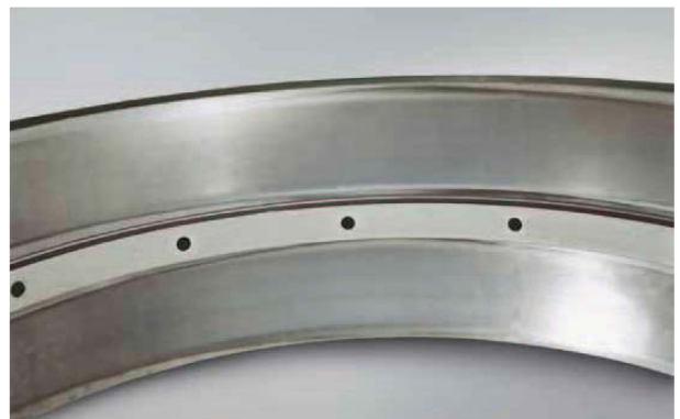
Photo 8.2 Part: Outer ring of a double-row tapered roller bearing Symptom: Indentations on raceway surface Cause: Debris caught in the surface
