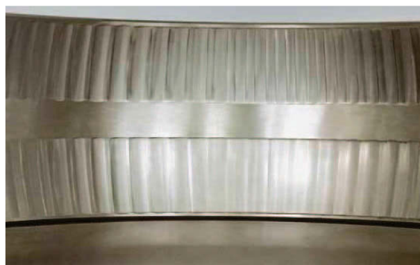
Photo 10.2 Part: Outer ring of a spherical roller bearing Symptom: Wear having a wavy or concave-and-convex texture on loaded side of raceway surface Cause: Entry of debris under repeated vibration while stationary
