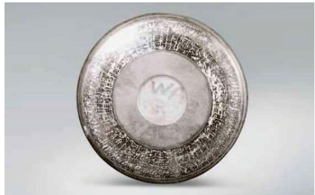
Photo 6.2 Part: Roller of a tapered roller thrust bearing Symptom: Thermal cracks occur at large end face of roller Cause: Heat generation due to sliding with the inner ring rib under poor lubrication
