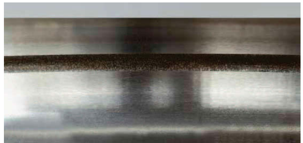
Photo 16.2 Part: Outer ring of a slewing ring Symptom: Rust on raceway surface at ball pitch Cause: Moisture condensation during stationary periods
