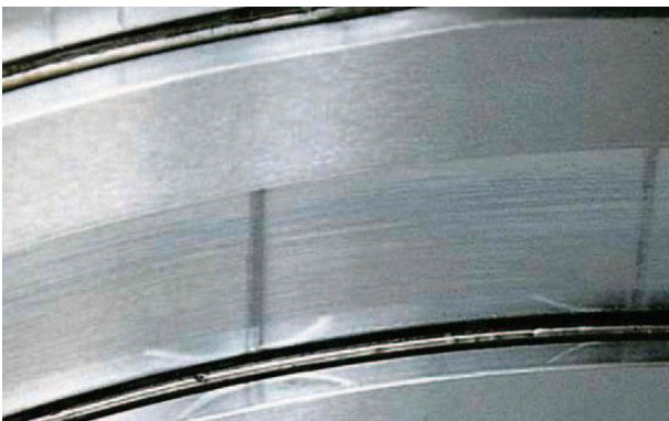
Photo 11.3 Part: Outer ring of a double-row cylindrical roller bearing Symptom: Fretting occurs on the raceway surface at roller pitch intervals
