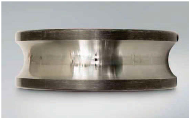
Photo 12.1 Part: Inner ring of a deep groove ball bearing Symptom: False brinelling occurs on the raceway Cause: Vibration from an external source while stationary
