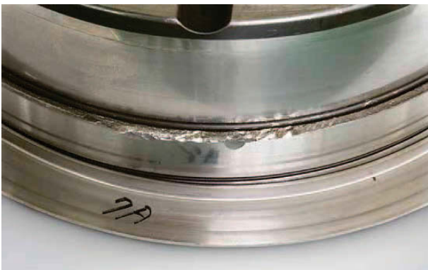
Photo 5.1 Part: Inner ring of a double-row cylindrical roller bearing Symptom: Chipping occurs at the center rib Cause: Excessive load during mounting
