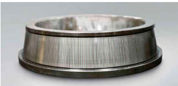
Photo 15.1 Part: Inner ring of a tapered roller bearing Symptom: Striped pattern of corrosion occurs on the raceway surface
