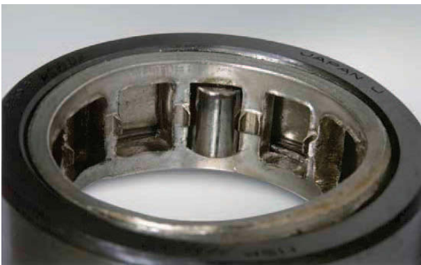
Photo 7.7 Part: Cage of a cylindrical roller bearing Symptom: Deformation and wear of a machined high-tension brass cage
