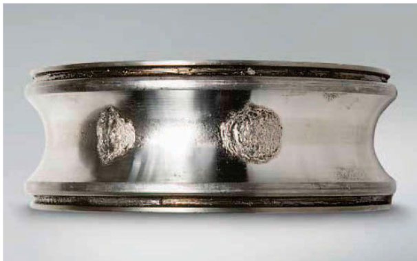
Photo 1.3 Part: Inner ring of deep groove ball bearing Symptom: Flaking of raceway at ball pitch Cause: Dents due to shock load during mounting
