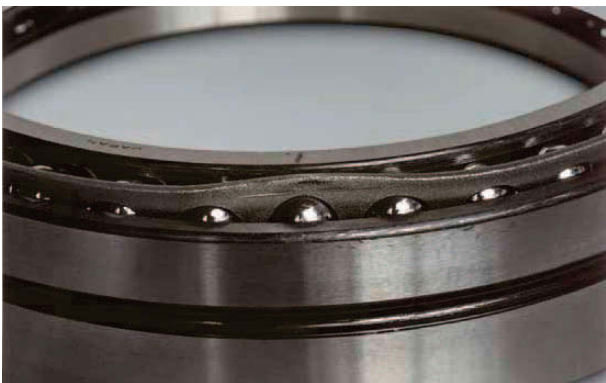
Photo 7.5 Part: Cage of an angular contact ball bearing Symptom: Pressed-steel cage deformation Cause: Shock load due to poor handling
