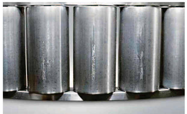
Photo 1.10 Part: Rollers of a cylindrical roller bearing Symptom: Premature flaking occurs axially on the rolling surfaces Cause: Scratches caused during improper mounting
