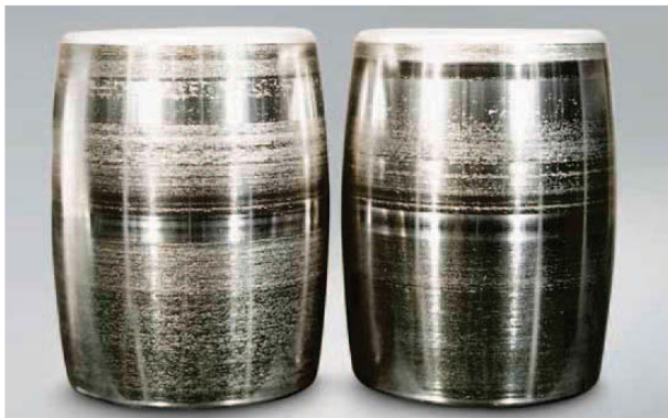
Photo 4.7 Part: Convex rollers of Photo 4.5 Symptom: Smearing occurs at the center of the rolling surface Cause: Poor lubrication
