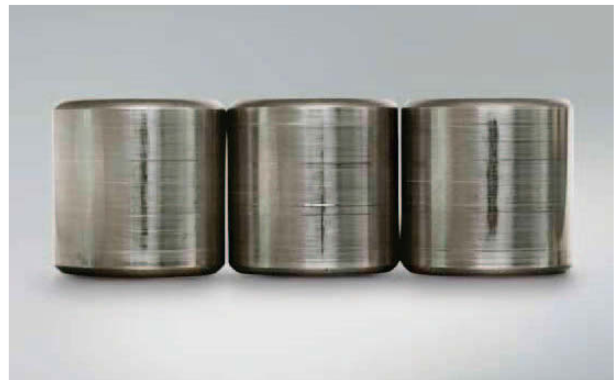
Photo 12.4 Part: Rollers of a cylindrical roller bearing Symptom: False brinelling occurs on rolling surface Cause: Vibration from an external source while stationary
