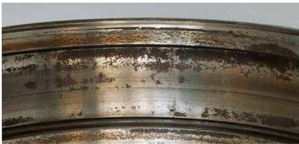
Photo 16.1 Part: Outer ring of a cylindrical roller bearing Symptom: Rust on the rib face and raceway surface Cause: Poor lubrication due to water entry
