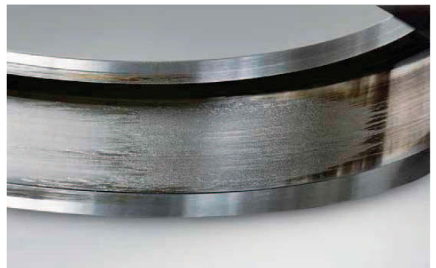
Photo 4.2 Part: Outer ring of Photo 4.1 Symptom: Smearing occurs circumferentially on raceway surface Cause: Roller slipping due to excessive grease filling
