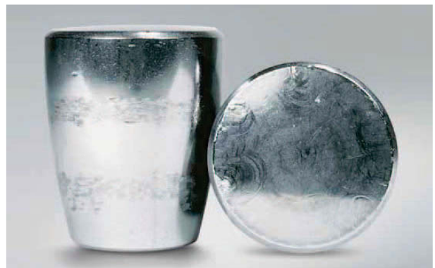
Photo 3.6 Part: Convex rollers of Photo 3.5 Symptom: Scoring on the roller end face Cause: Debris, which is caught in surface, and excessive axial loading
