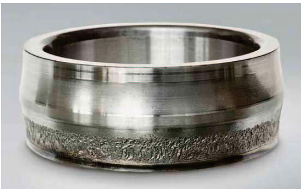
Photo 1.7 Part: Inner ring of a spherical roller bearing Symptom: Flaking of only one raceway over its entire circumference Cause: Excessive axial load
