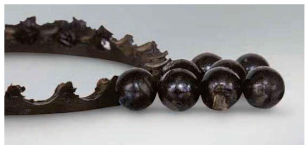
Photo 14.5 Part: Balls and cage of Photo 14.3 Symptom: Cage is damaged by melting, balls become discolored and melted Cause: Excessive preload
