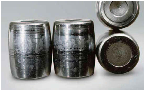
Photo 2.3 Part: Convex rollers of Photo 2.1 Symptom: Round shaped peeling pattern occurs on the center of the rolling surfaces Cause: Poor lubrication
