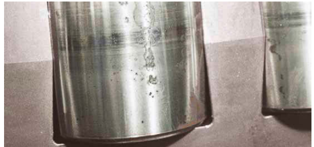
Photo 16.4 Part: Rollers of a spherical roller bearing Symptom: Pit-shaped rust on rolling contact surface. Corroded portions. Cause: Moisture condensation during storage
