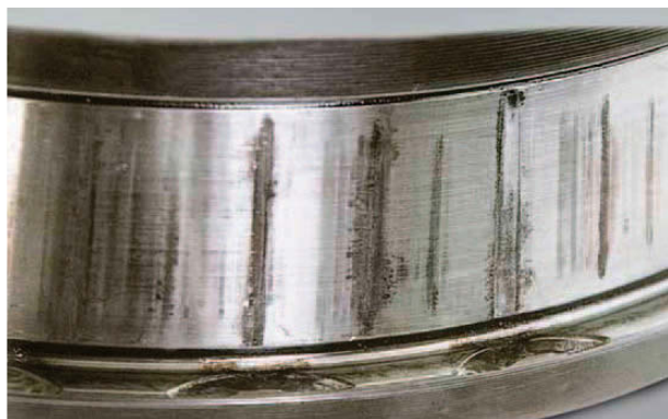
Photo 10.3 Part: Inner ring of a double-row tapered roller bearing Symptom: Fretting wear of raceway and stepped wear on the rib face Cause: Fretting progression due to excessive load while stationary
