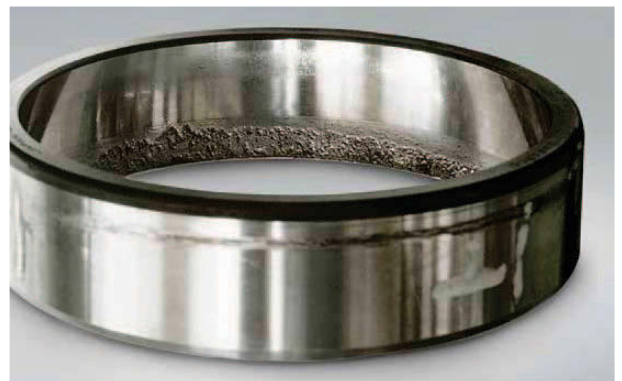
Photo 1.8 Part: Outer ring of Photo 1.7 Symptom: Flaking of only one raceway over its entire circumference Cause: Excessive axial load
