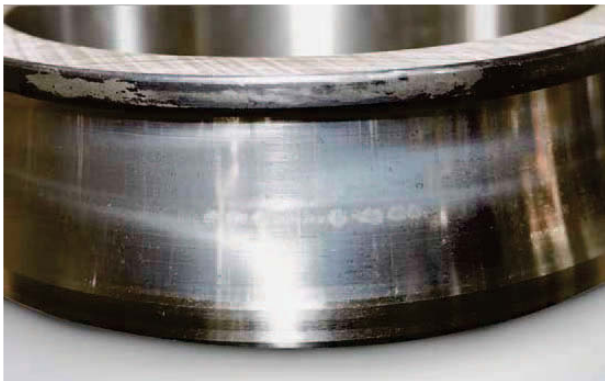
Photo 2.1 Part: Inner ring of a spherical roller bearing Symptom: Round shaped peeling pattern occurs on the center of the raceway surface Cause: Poor lubrication
