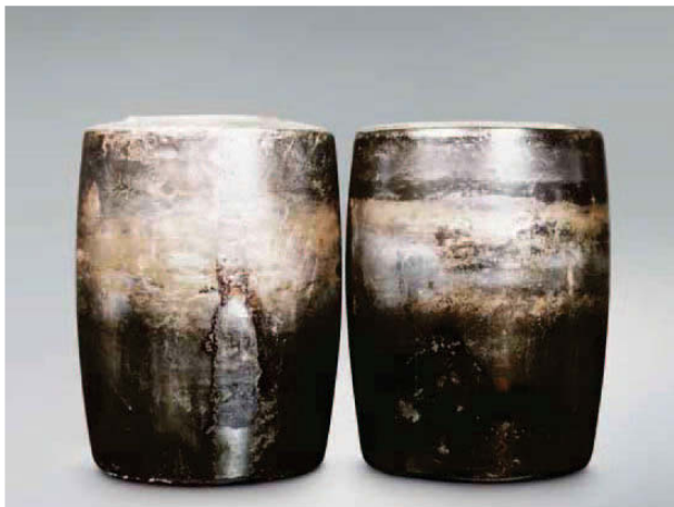
Photo 14.2 Part: Convex rollers of Photo 14.1 Symptom: Discoloration and melting of roller rolling surface, adhesion of worn particles from cage Cause: Insufficient lubrication
