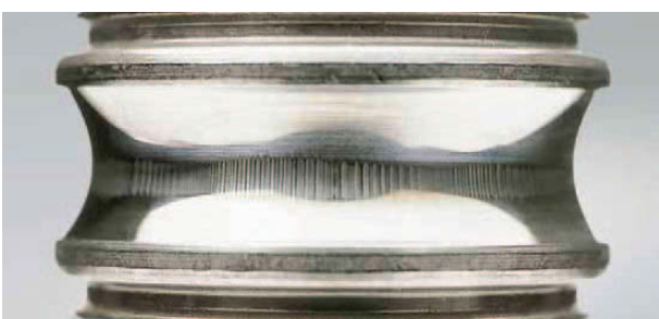
Photo 15.5 Part: Inner ring of a deep groove ball bearing Symptom: Fluting occurs on the raceway surface (High frequency)
