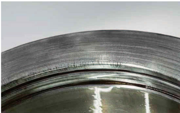
Photo 6.1 Part: Outer ring of a double-row cylindrical roller bearing Symptom: Thermal cracks occur on the outer ring side face Cause: Abnormal heat generation due to contact sliding between mating part and face of outer ring
