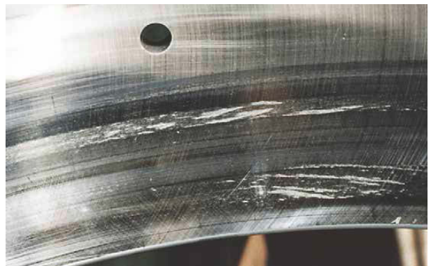
Photo 4.6 Part: Outer ring of Photo 4.5 Symptom: Partial smearing occurs circumferentially on raceway surface Cause: Poor lubrication
