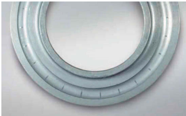
Photo 12.3 Part: Outer ring of a thrust ball bearing Symptom: False brinelling of raceway surface at ball pitch Cause: Repeated vibration with a small oscillating angle
