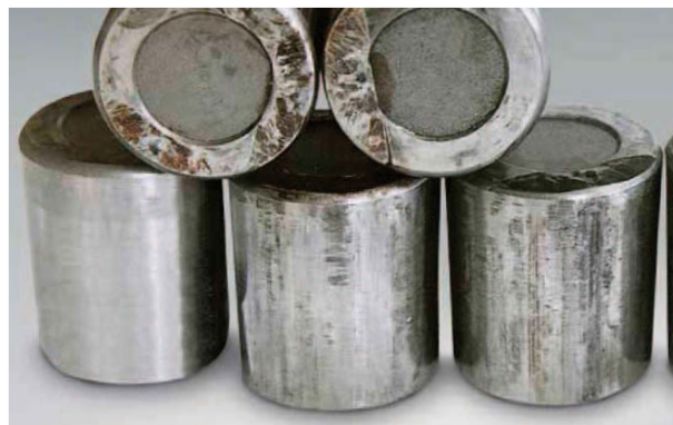
Photo 10.4 Part: Tapered rollers of Photo 10.3 Symptom: Stepped wear on the roller head and face Cause: Fretting progression due to excessive load while stationary
