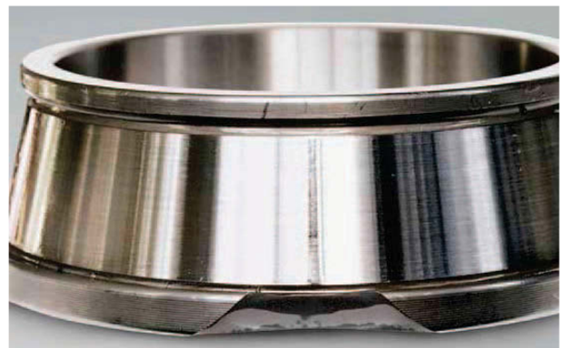
Photo 5.2 Part: Inner ring of a tapered roller bearing Symptom: Fracture occurs at the cone back face rib Cause: Large shock during mounting
