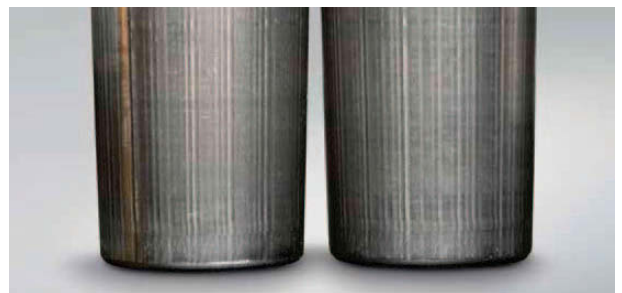
Photo 15.2 Part: Tapered rollers in Photo 15.1 Symptom: Striped pattern of corrosion occurs on the rolling surface
