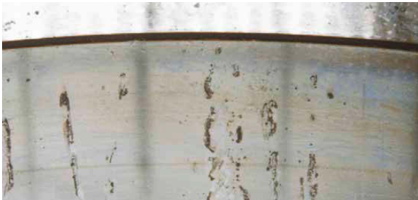
Photo 16.3 Part: Inner ring of a spherical roller bearing Symptom: Rust on raceway surface at roller pitch Cause: Entry of water into lubricant
