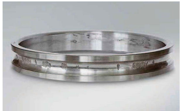
Photo 1.4 Part: Inner ring of an angular contact ball bearing Symptom: Flaking of raceway at ball pitch Cause: Dents due to shock load while stationary
