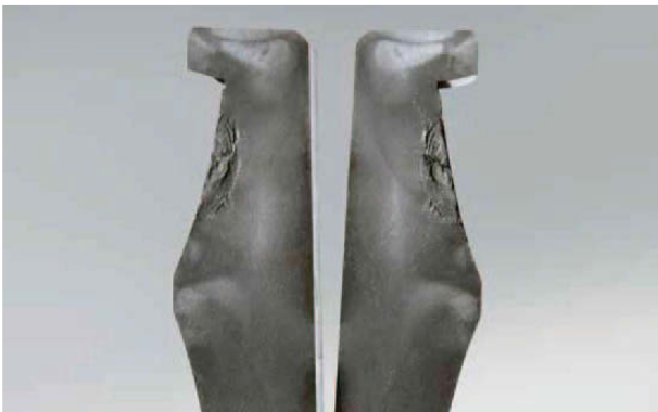
Photo 6.7 Part: Cross section of a fractured inner ring in Photo 6.6 Symptom: Origin is directly beneath the raceway surface
