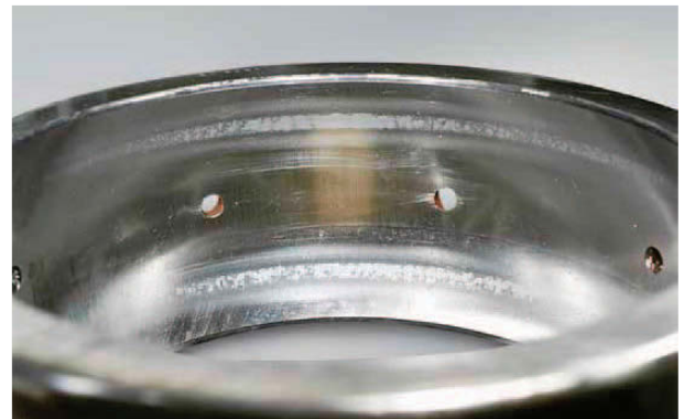
Photo 2.4 Part: Outer ring of a spherical roller bearing Symptom: Peeling occurs near the shoulder of the raceway over the entire circumference Cause: Poor lubrication
