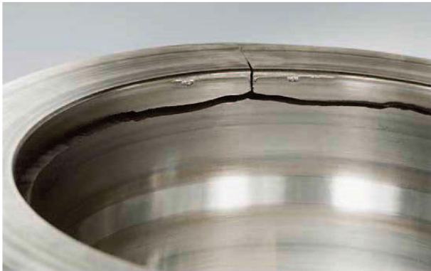
Photo 6.3 Part: Outer ring of a double-row cylindrical roller bearing Symptom: Cracks propagated outward in the axial and circumferential directions from the flaking origin on the raceway surface Cause: Flaking from a flaw due to shock
