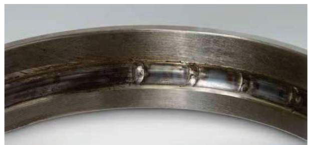
Photo 14.4 Part: Outer ring in Photo 14.3 Symptom: Raceway discoloration, melting occurs at ball pitch intervals Cause: Excessive preload
