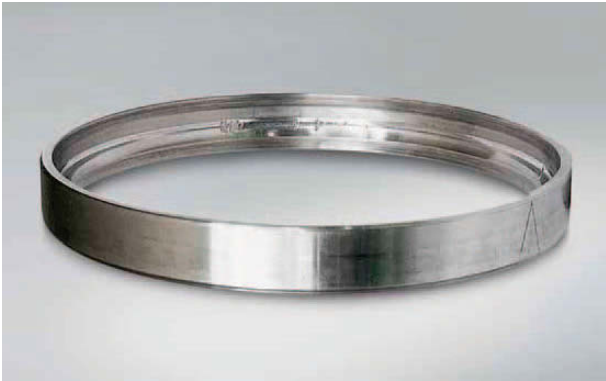
Photo 1.5 Part: Outer ring of Photo 1.4 Symptom: Flaking of raceway surface at ball pitch Cause: Dents due to shock load while stationary
