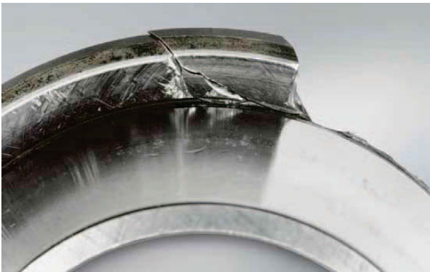
Photo 5.3 Part: Inner ring of a spherical thrust roller bearing Symptom: Fracture occurs at the large rib Cause: Repeated load
