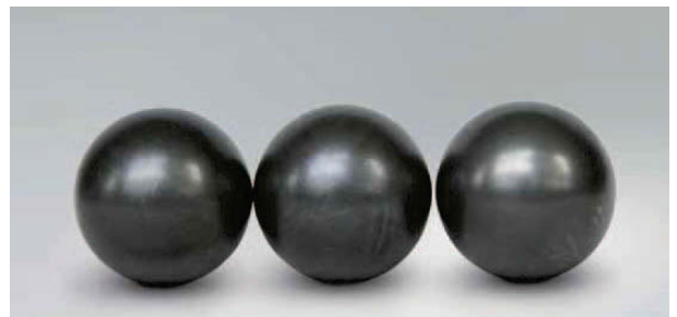
Photo 15.4 Part: Balls of a groove ball bearing Symptom: Electrical corrosion has a dark color that covers the entire ball surface
