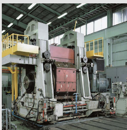
Test rig for bearings used in backup rolls of rolling mills
